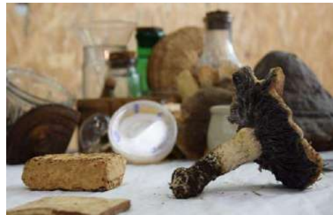
Mushrooms to stop plastic pollution. Cultivating mycelium mixed with agricultural waste enables the creation of a sturdy and completely biodegradable packaging material.
